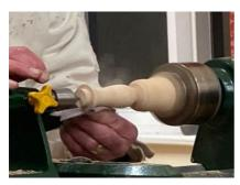
Once sanded to 320 grit, Dave drilled into the handle from the thread end to take the darning needles. The handle was finished in the same way as the mushroom cap and parted off.
