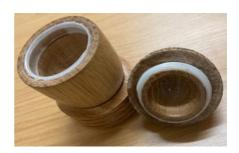
Removing the thread from the bottle is best done by first rough-cutting the body of the bottle away, mounting the opening on to a jam chuck and using a Stanley knife to cut upwards into the spin of the lathe. Use the same technique to remove the flat top from the cap leaving only the thread. Caution should be taken to check the bottles are not too brittle.
