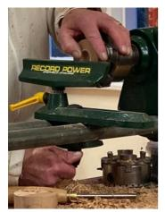
The mushroom head was then reversed on to a pin chuck to finish the top. Sanded through the 320 grit and finished with Microcrystalline polish. Hard polishes are recommended for items that will be handled although they do tend to leave a white residue in open grained wood. Ideally leave
